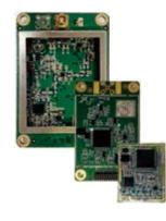
SDL series modules are SOUTH's self-developed internal digital radio which are built for mission-critical applications where a combination of flexibility and supreme performance, which can fully support the communications with the mainstream radio protocols such as Trimtalk450S, SOUTH, SOUTH+, SOUTHx, huace, ZHD and Satel. Realize the random switching of the radio range 410MHz-470MHz in any channels and the power level as well.
