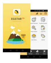
EGStar for Android is designed for old users by remaining classical menus which is similar to the previous version on Windows Mobile platform, and also for new users with popular Android interface at present, these 2 user interfaces are able to be switched according to the operation habit of users.
