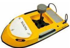
SOUTH SL20 surveying boat adopts dual spray pumps for the propulsion system, and use differential motion to control driving direction of boat. This propulsion system greatly improve the disadvantages of propeller system in previous products that in case of aquatic plants are sucked into propeller and damage the propulsion system.
