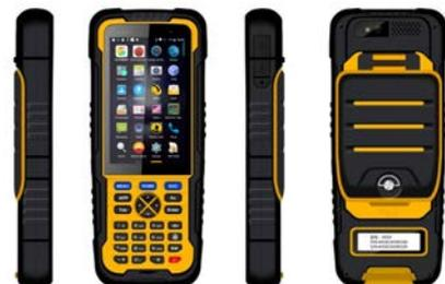
H3 plus is a new generation professional controller running on Android which offers state of the art smartphone capabilities combined with rugged professional quality. And the alphanumeric keypad which gives flexibility for surveyors field work.
