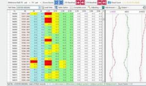
Raw ride performance data of track detection (unadjusted) and statistical analysis results before adjustment
