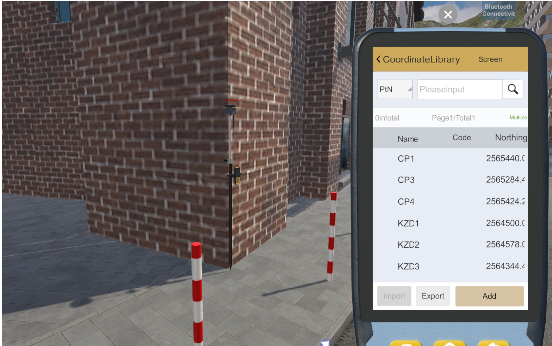
Figure 3: Rover is connected to controller during survey work
