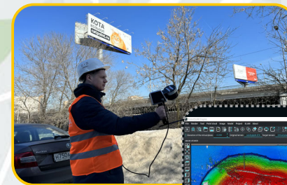
Stockpile Volume Calculation RobotSLAM in handheld mode, Russia
