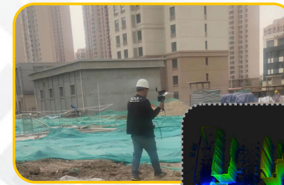
Building As-built Survey RobotSLAM in handheld mode, China
