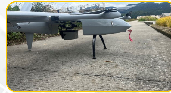
Countryside Topography 1:500, VTOL fixed-wing + LiDAR, China
