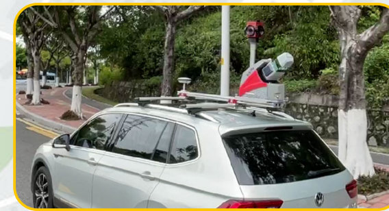
High-precision Street Mapping, SUV-based LiDAR + 360° Pano Camera, China
