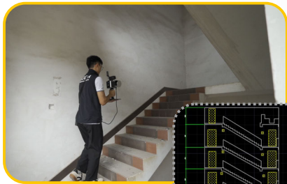
Building Elevational Surveying RobotSLAM in handheld mode, China
