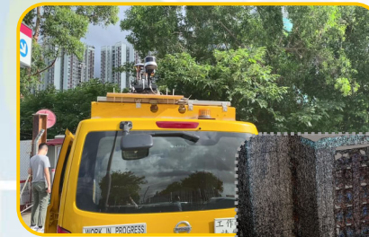
Road Inventory E-documentation RobotSLAM in SUV-based mode, Hong Kong
