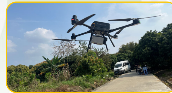
Power Grid Inspection, UAV-based LiDAR + RGB Camera, China
