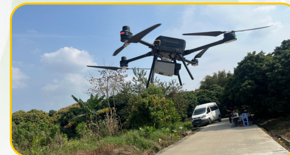
Power Grid Inspection, UAV-based LiDAR + RGB Camera, China
