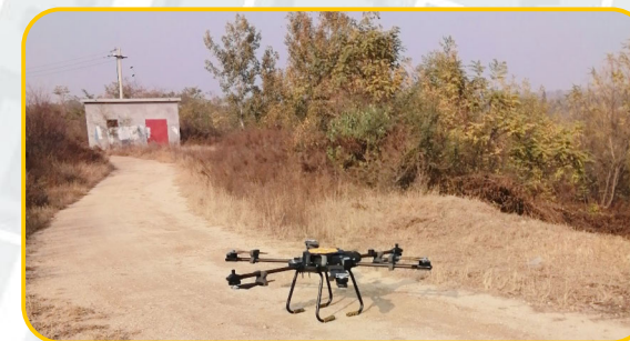
Reservoir Topography 1:500, UAV-based LiDAR + RGB Camera, China
