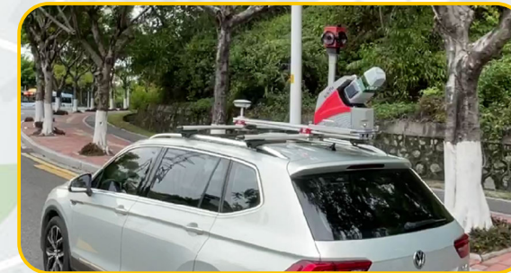
High-precision Street Mapping, SUV-based LiDAR + 360° Pano Camera, China
