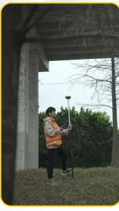
**RTK Receiver RTK Receiver**
