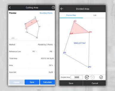
Select points to form a polygon, and directly identify the area division points for the surveyor to stake out. There is no more need for the user to guess a position to measure, and then to adjust.
