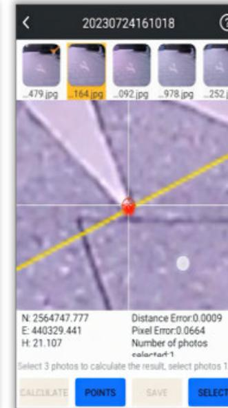
Photogrammetry Measurements can be conducted by taking pictures or videos. Coordinates of all points in the photos can be acquired.
